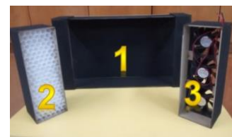
Gambar 4.22. (1) test section , (2) honeycomb , (3) fan
